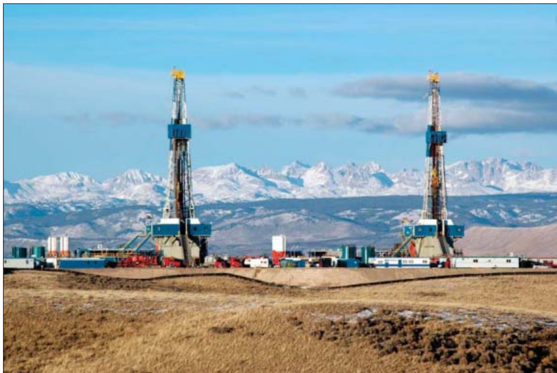
Well spacing at Pinedale ranges from 40 to 5 acres, with many wells drilled deviated from well pads that accommodate multiple wellheads and minimize the drilling and production footprint (Fig. 3). Photo from Shell.
