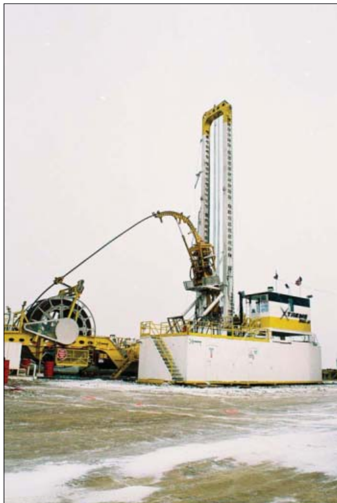
Xtreme's CT Rig 2, model 200ST, was drilling near Rock Springs, Wyo., in late 2006 for Shell Unconventional Resources (Fig. 1; photo from Tenaris Coiled Tubes and Xtreme Coil Drilling Corp.).
